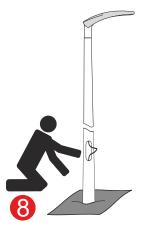
Connect the power cable to the power supply.
