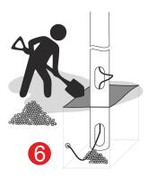
Cover up the pit with native soil, thickening it layer by layer with a mechanical earth rammer.
