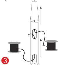
Insert the power cable into the bottom hole of the column and pass it all the way up to the column finial.
