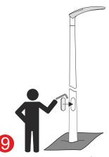
Screw the inspection flap using an Allen key. The column is ready to use.
