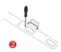
Unscrew the inspection flap of the composite column.
