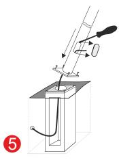
Unscrew the inspection flap and pass the cable through it. Place the column onto the precast base. Use the supplied screws, washers and blind nuts to attach the column foot.
