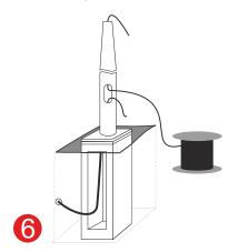
Insert the power cable of the LED luminaire into the hole of the inspection flap and pass it all the way up to the column finial.
