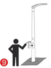
Screw the inspection flap using an Allen key. The column is ready to use.
