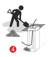
Cover up the pit with native soil, thickening it layer by layer with a mechanical earth rammer.
