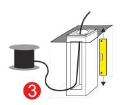
Put the precast base upright and make sure it is perfectly level. Insert the power cable into the hole in the precast base.
